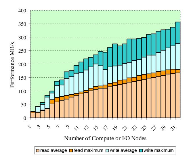
The performance of SFIO over MPI-FCI is measured for concurrent access from all compute nodes to all I/O nodes. In order to limit operating system caching effects, the total size of the striped file linearly increases with the number of I/O nodes up to 32GB. The stripe unit size is 200 bytes. The MPI-FCI application's I/O performance is measured as a function of the number of Compute and I/O nodes. For each configuration, 53 measurements are carried out.
