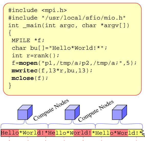
Multiple compute nodes accessing a striped file. The striped file with a stripe unit size of 5 bytes consists of two subfiles.
