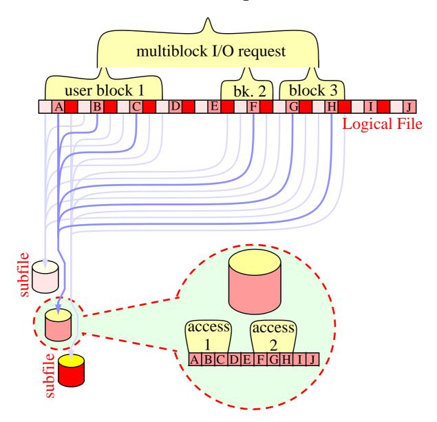
SFIO merges several disk accesses into a single disk access request. The algorithm implemented on the compute node tries to combine all overlapping or consecutive I/O requests. The 6 original data segments to be accessed are grouped into 2 remote subfile requests.
