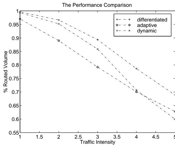
Fig. 2. Percent routed volume performance comparison of adaptive, dynamic, and differentiated shortest path routing.
