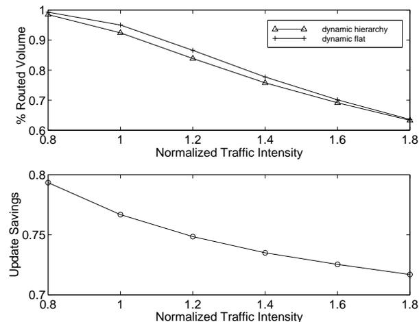
Fig. 5. Percent routed volume comparison (top) and update savings (bottom) achieved by the effective resistance hierarchical routing.
