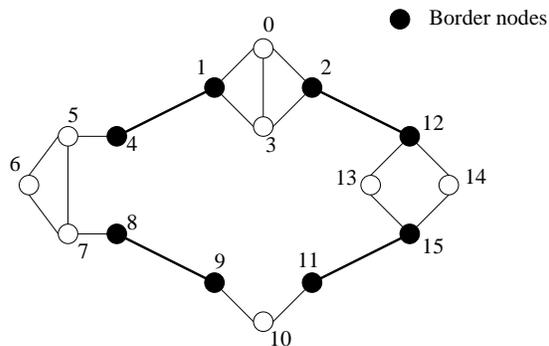
Fig. 4. A 2-level hierarchical network.
