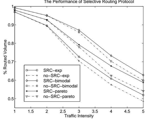
Fig. 3. Performance achieved with and without the selective routing control for heterogeneous user demands.
