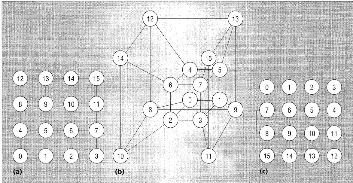
Figure 5. Network topologies: (a)  $4 \times 4$  mesh; (b) 4D hypercube; (c) linear array.
