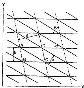
FIG. 1. Diagram of moiré fringes (dotted lines of spacing  $d$ ) produced from two linear parallel rulings (spacing  $a$  and  $b$ ). Note  $AB^2 = AC^2 + BC^2 - 2AC \times BC \cos\theta$ , and since area of  $ABCD = AB \times d = AC \times a = BC \times b$  then  $d^2 = a^2 + b^2 - 2a^{-1}b^{-1} \cos\theta$ .
