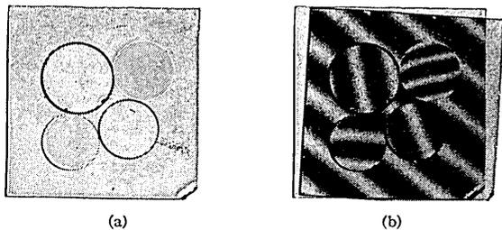
FIG. 5. Moiré patterns for lenses. (a) Figure produced by lenses placed on a regular ruling (upper left: plano convex  $f=81$  mm, upper right: meniscus  $f=-76$  mm, lower left: meniscus  $f=-36$  mm, lower right: plano convex  $f=114$  mm). (b) Moiré patterns produced by overlapping regular rulings on (a). Patterns for combinations of two lenses are achieved by placing the second lens on the appropriate portion of (a) and viewing through the regular rulings.
