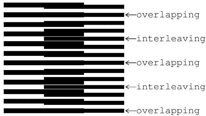
Figure 2. Superposition of two layers consisting of horizontal parallel lines [eps], [tif], [png]
