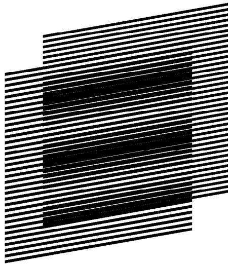
Figure 6. Superposition of layers consisting of inclined parallel lines where the lines of the base and revealing layers are inclined at the same angle [eps], [png]
