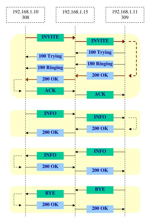
During the phone conversation there are two transactions with INFO messages. These transactions correspond to transmissions of DTMF signals via SIP messages. The first INFO message tells that the digit "2" is pressed on the calling phone for 4800 milliseconds. The second INFO message tells that the digit "3" is pressed on the called phone for 480 milliseconds. To make sure that SIP INFO messages are transmitted, we must specify the transmission of DTMF signals with SIP messages to SIP phones:
