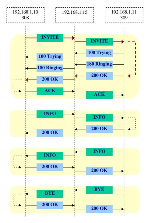
During the phone conversation there are two transactions with INFO messages. These transactions correspond to transmission of DTMF signals via SIP messages. The first INFO message tells that the digit "2" is pressed on the calling phone for 4800 milliseconds. The second INFO message tells that the digit "3" is pressed on the callee phone for 480 milliseconds. To make sure that SIP INFO messages are transmitted, we must specify in SIP phones the transmission of DTMF signals with SIP messages:
